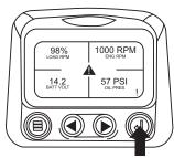
Touching the "Enter Button" once again will hide the fault and return the screen to the single or four parameter display.
